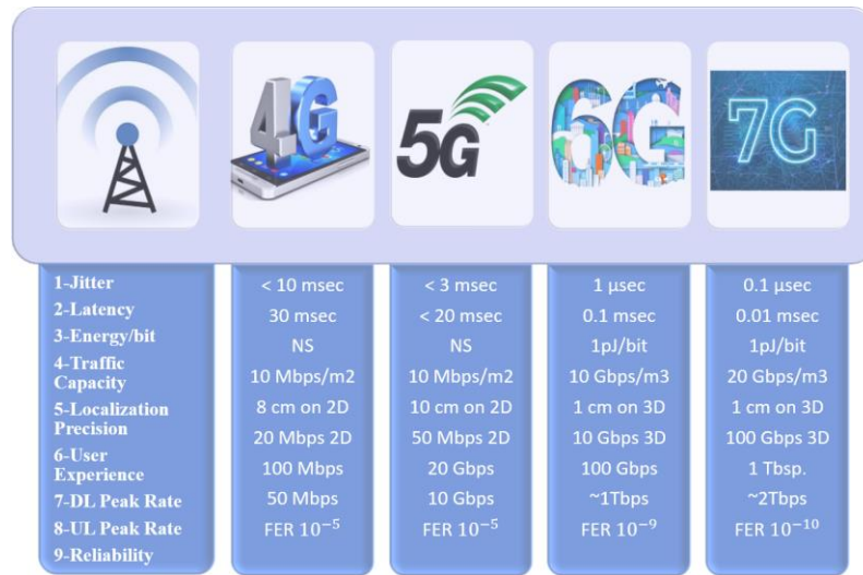
Figure 4: The Technical Specifications for Latency, Jitter, and Data Rates from 4G to a Hypothetical 7G (Vaigandla et al., 2021; Zontou, 2023; Takehiro, 2009 & "What is Jitter, Wander and Latency," 2023)
