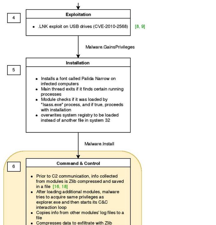
Figure 14: Gauss Kill Chain Diagram Part 2, illustrating steps 4,5 and 6
