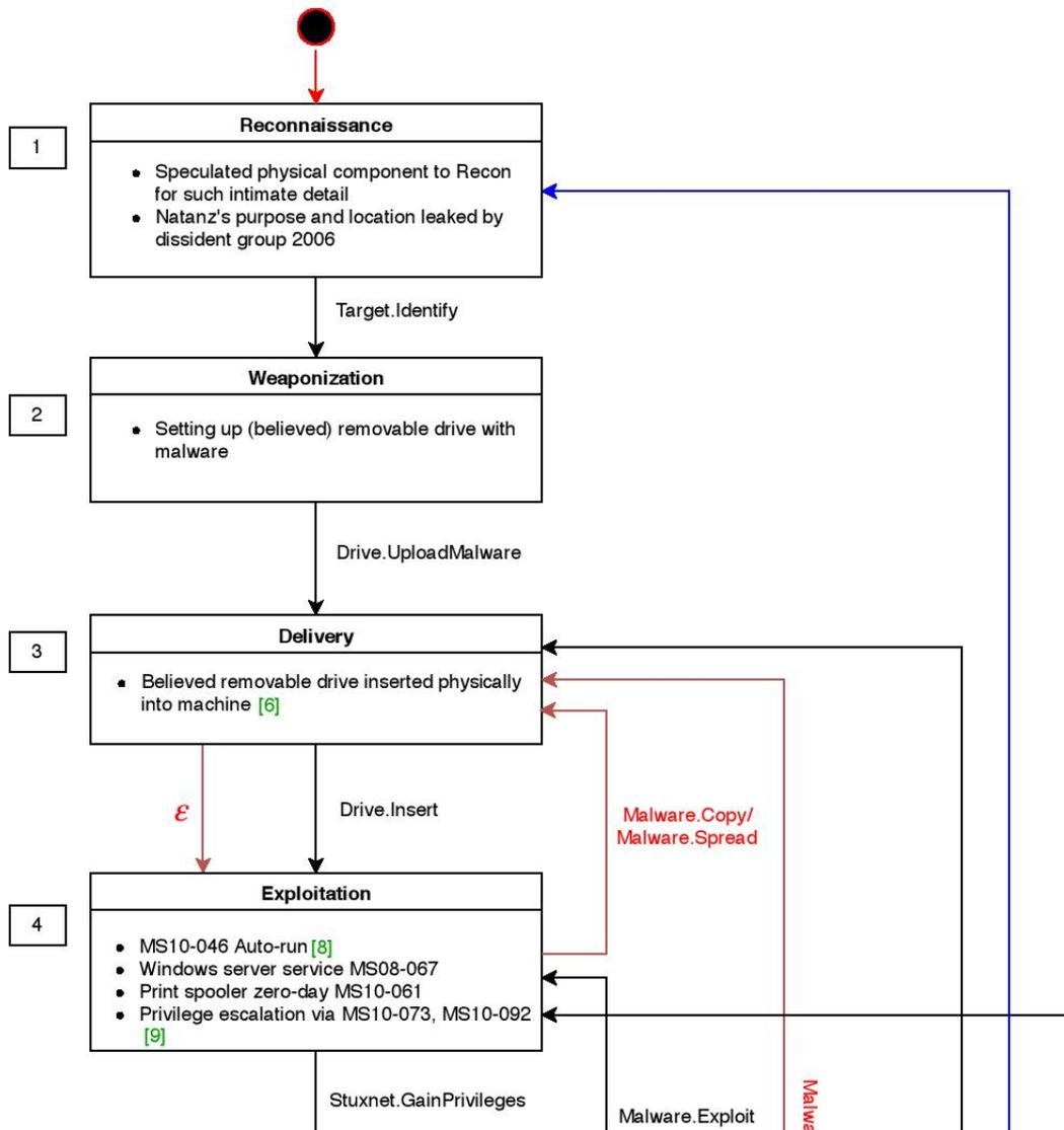
Figure 1: Stuxnet Verbose Diagram Part 1 detailing steps 1, 2, 3 and 4 of the Kill Chain
