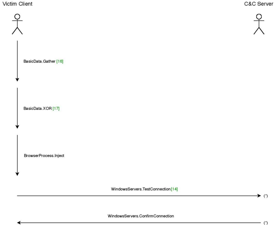
Figure 5: Stuxnet MSQ Diagram Part 1
