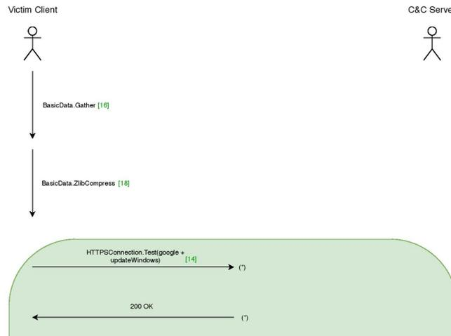
Figure 18: Gauss MSQ Diagram Part 1
