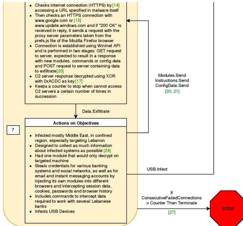
Figure 15: Gauss Kill Chain Diagram Part 1, illustrating step 7
