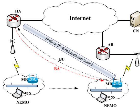
Figure 1: Architecture of NEMO-BSP
