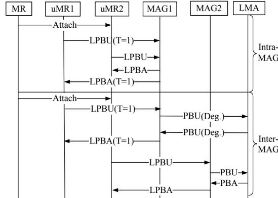
Figure 6: Handover procedure of N-NEMO
