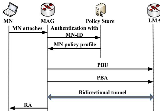
Figure 2: Signaling call flow of basic PMIPv6
